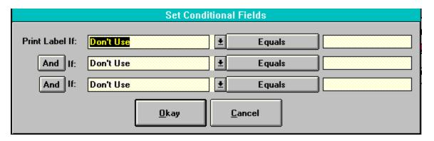
You can set up to three **Conditional Sentences** that filter the printing of labels from a database in *ViaPrint*.
