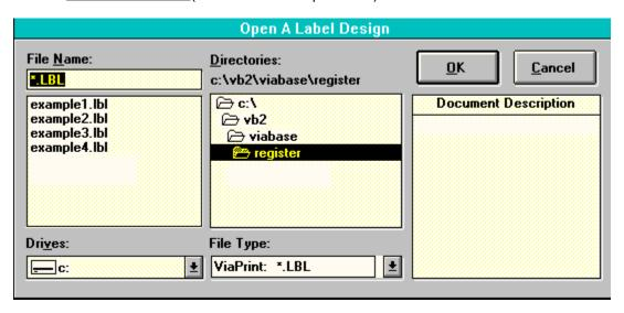
Use this function to load a previously saved label into *ViaPrint* for editing or printing. Select the label you wish to load from the list of files on the File Window that will appear and press "OK".
